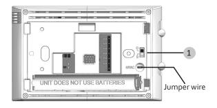
**Instructions:** To convert the system from PTHP to PTAC, cut the jumper wire located on the back of the thermostat. Change menu item #20 from default HP to AC.
