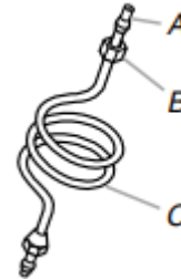
A. Compression sleeve B. Compression nut C. Copper tubing
