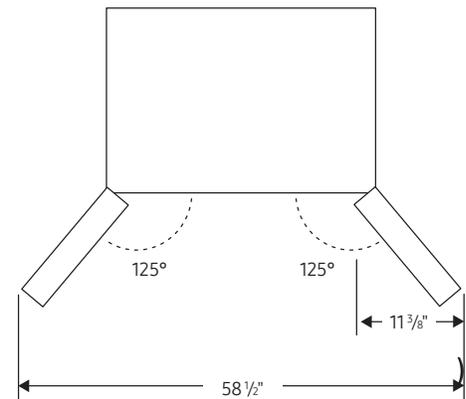
NOTE: Please allow  $3\frac{3}{4}"$  of clearance when installing along a wall.
