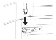
2 Fit the hinge 10 over the hinge lever latch 2 and slot it into place. Rotate the lever 3 clockwise and fasten the hinge.
