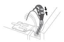
4 Push the water supply lines into the hole on the top case and pull it through the backplate.
