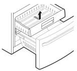
4 Remove the Durabase basket from the rails. Remove the screws from the rails at both ends.
