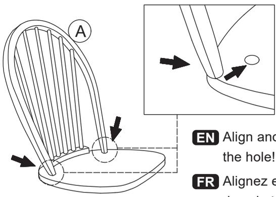
**EN** Align and press into the hole!
