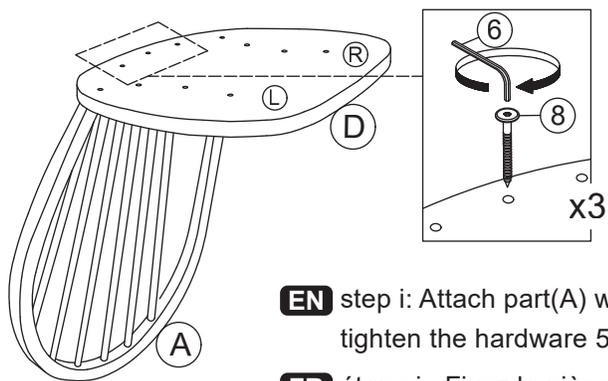
**EN** step i: Attach part(A) with part(D), tighten the hardware 50%!
