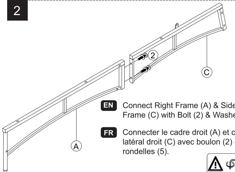
**EN** Connect Right Frame (A) & Side Right Frame (C) with Bolt (2) & Washers (5)
