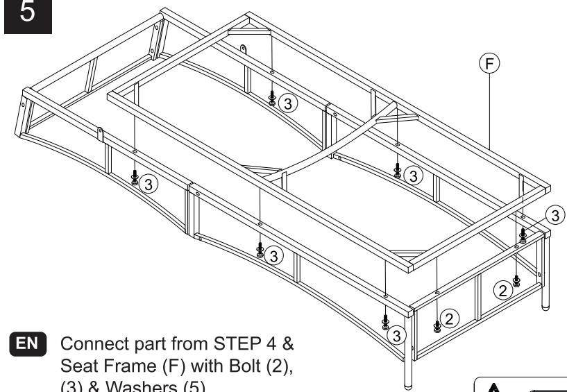
**EN** Connect part from STEP 4 & Seat Frame (F) with Bolt (2), (3) & Washers (5)
