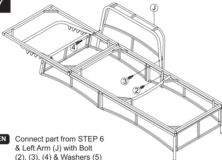
**EN** Connect part from STEP 6 & Left Arm (J) with Bolt (2), (3), (4) & Washers (5)
