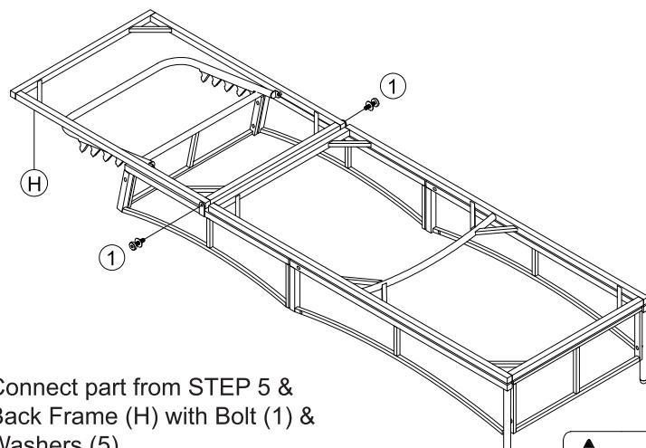
**EN** Connect part from STEP 5 & Back Frame (H) with Bolt (1) & Washers (5)
