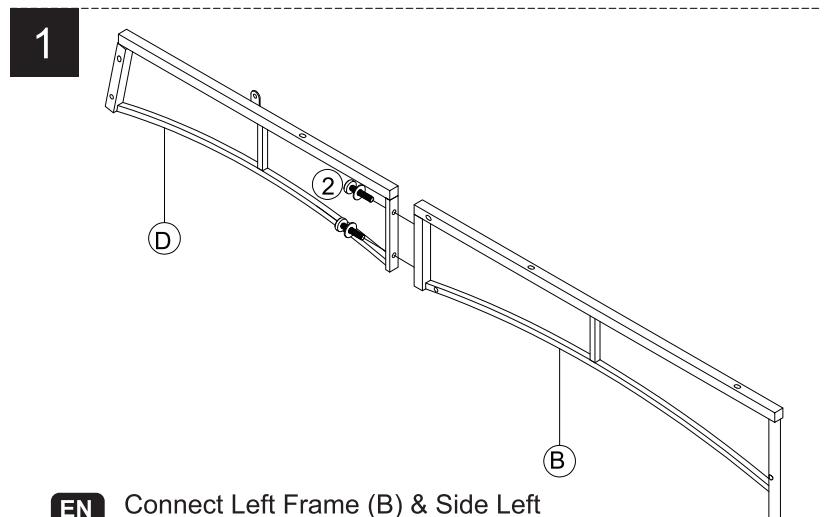
**EN** Connect Left Frame (B) & Side Left Frame (D) with Bolt (2) & Washers (5)
