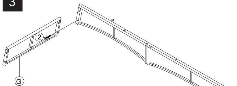
**EN** Connect part from STEP 1 & Front Frame (E) & Back side Frame (G) with Bolt (2) & Washers (5)
