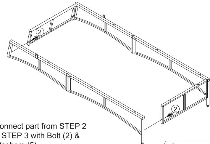
**EN** Connect part from STEP 2 & STEP 3 with Bolt (2) & Washers (5)
