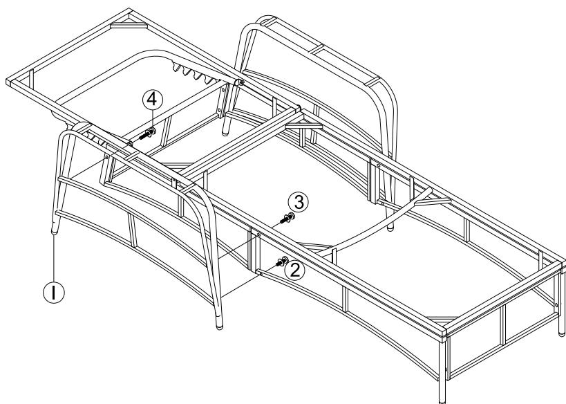
**EN** Connect part from STEP 7 & Right Arm (I) with Bolt (2), (3), (4) & Washers (5)
