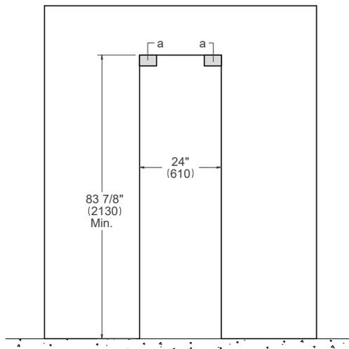
(a) Area to be left clear for the anti-tipping brackets – 3 1/2x5" (82x127mm)
