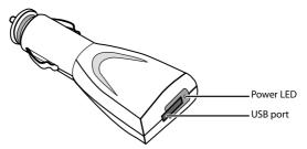
2 Plug the USB connector on the included USB cable into the USB port on the car adapter.
