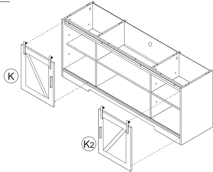
Place the two laminates on the support bracket
