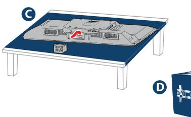
our TV has four VESA mounting noles on the back. If you attach a our TV, the bracket must be securely attached, using all fou
