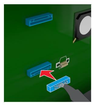
**c** Align the screws on the printer hard disk to the slots on the controller board bracket, and then slide the printer hard disk onto the brackets.
