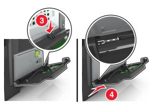
Run the ISP cable through the controller board shield.
