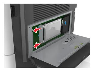
**d** Tighten the two screws.
