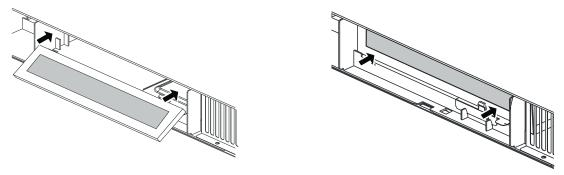
**6** Carefully push the vent grille back into place and replace the vent grille mounting screws.
