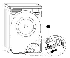
**2** Connect the drain hose of the dryer and secure the hose clamp.
