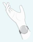
The Wave should be worn about an **inch away** from your hand with the **buttons facing** your elbow.
