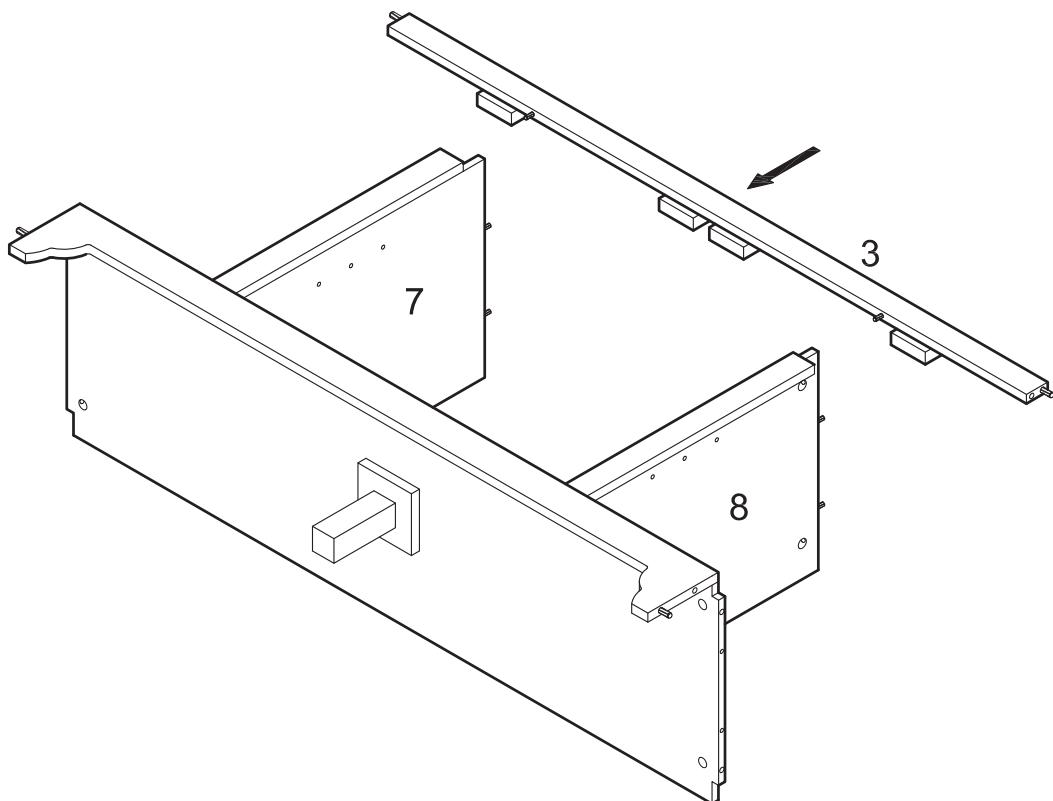
Attach slat (3) to panels (7,8) using dowels as guides.
