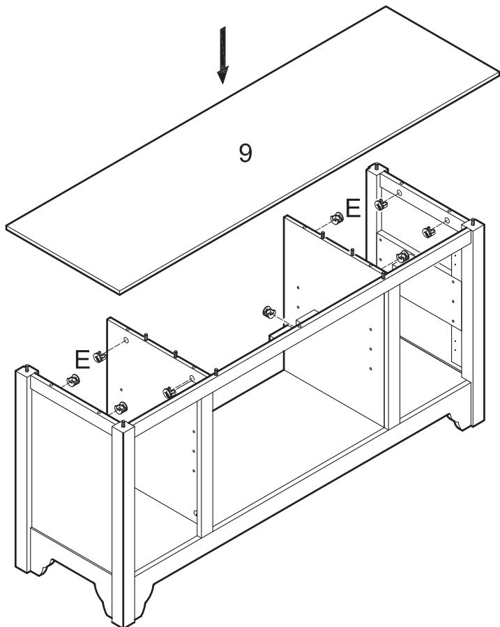
Insert cam locks (E) into the assembly from Step 9 as shown above. Attach top panel (9) to the assembly using cam bolts and dowels as guides. Tighten cam locks (E) with a screwdriver.
