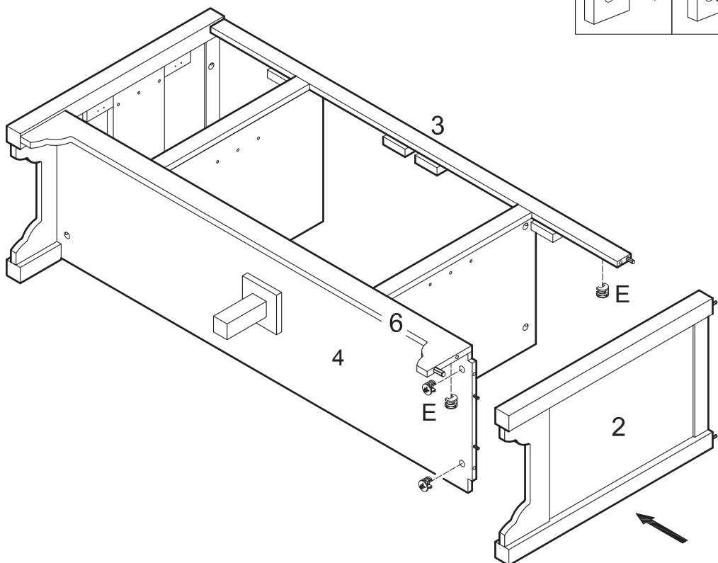
Attach side panel (2) to the opposite side of the assembly from Step 7 using cam bolts and dowels as guides. Insert cam locks (E) into bottom panel (4) and slats (3,6). Tighten cam locks (E) with a screwdriver.
