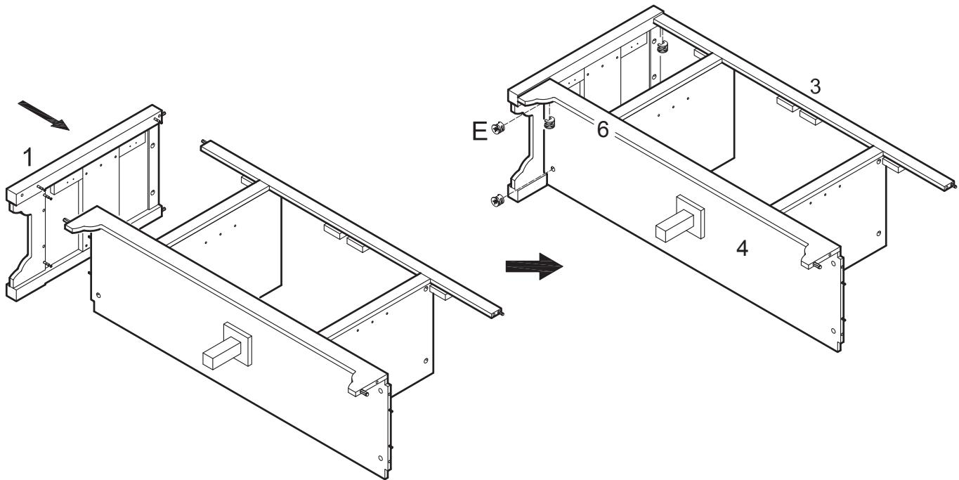
Attach side panel (1) to the assembly from the previous step using cam bolts and dowels as guides. Insert cam locks (E) into bottom panel (4) and slats (3,6). Tighten cam locks (E) with a screwdriver.
