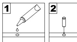
In future assembly steps when dowels are necessary to attach assembly parts together, place a small amount of glue on the end of the dowel before attaching parts together. Wipe away excess glue immediately.
