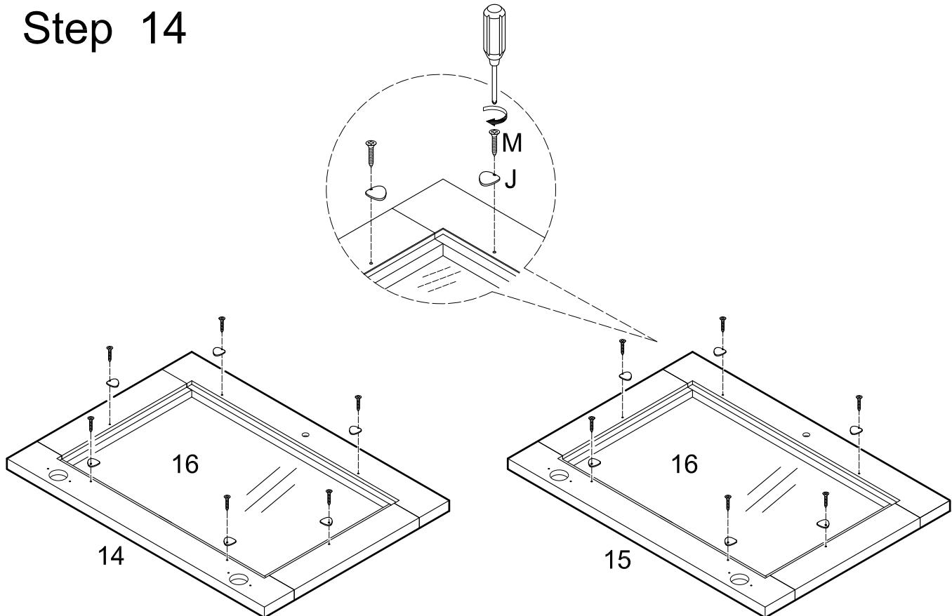
Secure glass panes (16) by attaching metal washers (J) to door frames (14,15) using screws (M). *The curve of metal washers (J) will arc into glass panes (16).*
