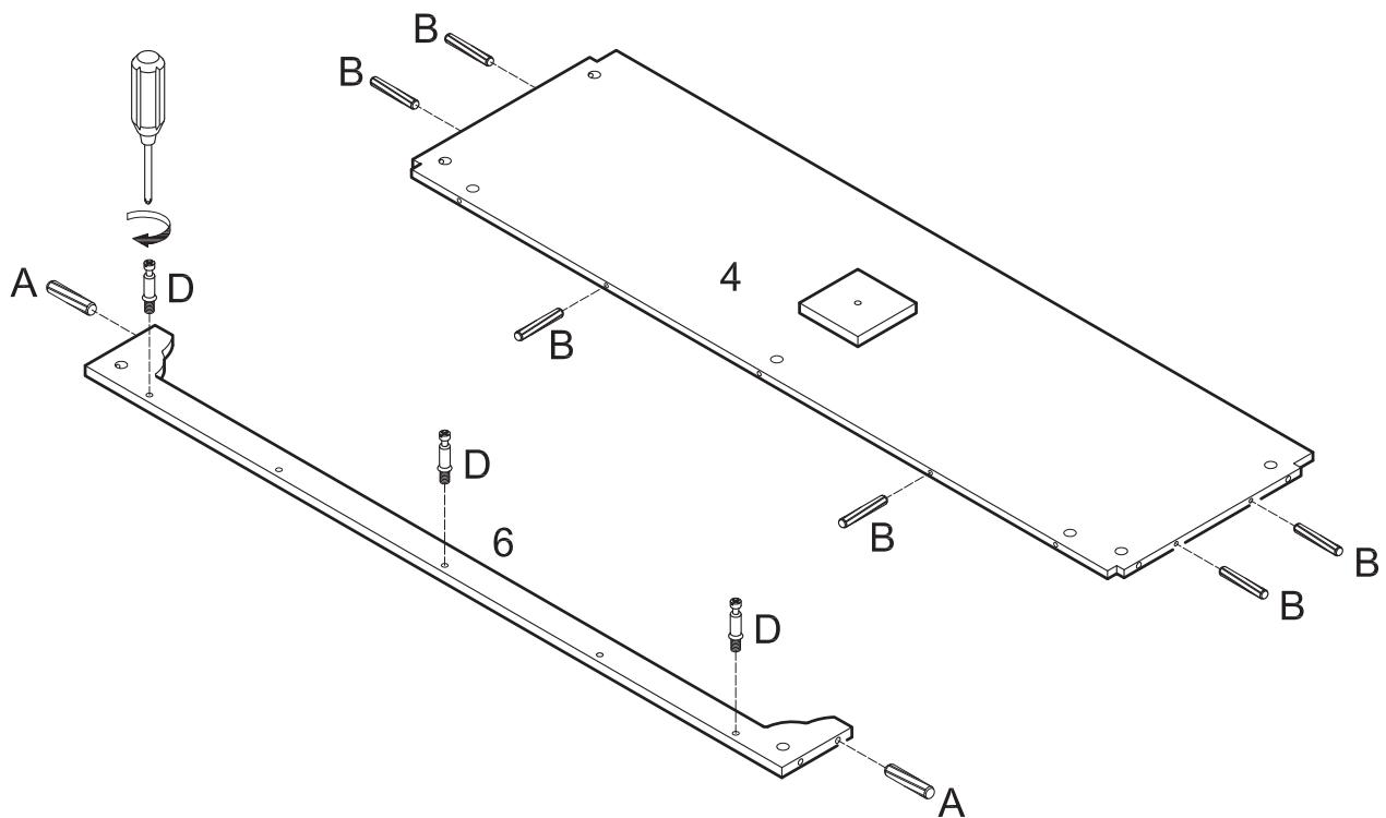
Insert large dowels (A) into slat (6). Insert small dowels (B) into bottom panel (4). Screw cam bolt (D) into slat (6).
