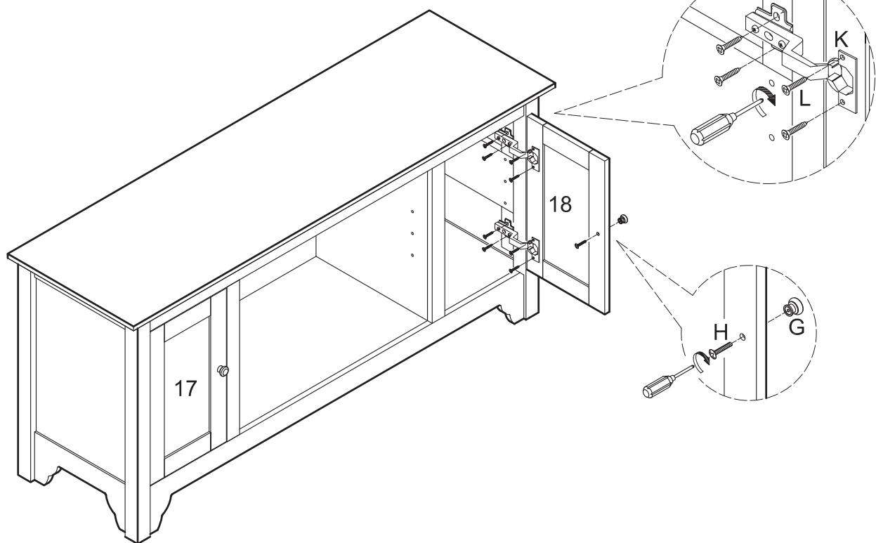
Attach hinges (K) to the interior of the assembly, then to doors (17,18) using screws (L). Attach handles (G) to doors (17,18) using bolts (H).
