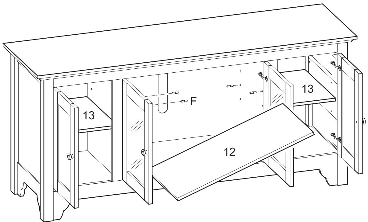
Insert shelf support pins (F) into the interior of the assembly at desired shelf heights. Carefully place shelves (12,13) on shelf support pins (F).
