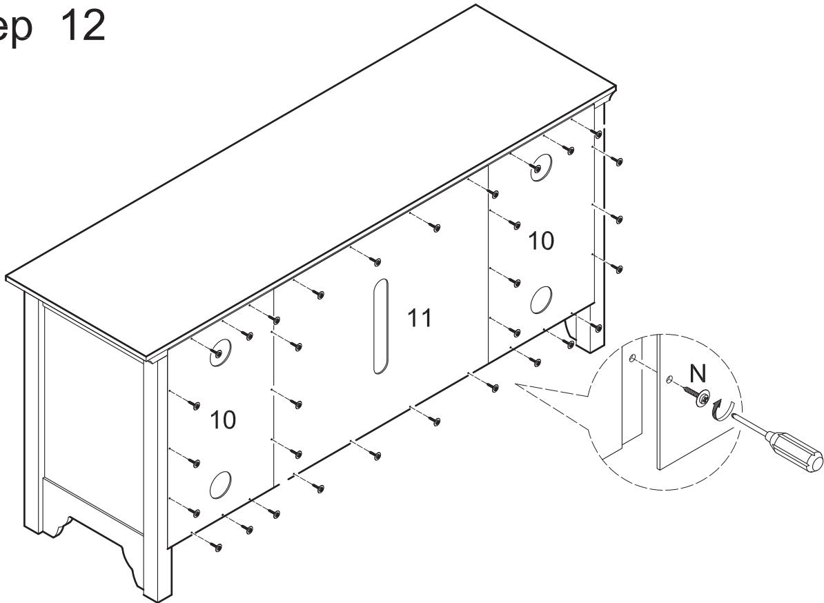
Attach back panels (10,11) to the assembly from the previous step using screws (N). Note that back panels (10) will overlap back panel (11).
