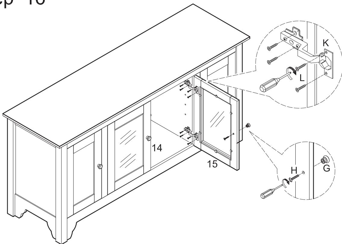
Attach hinges (K) to the interior of the assembly, then to doors (14,15) using screws (L). Attach handles (G) to doors (14,15) using bolts (H).
