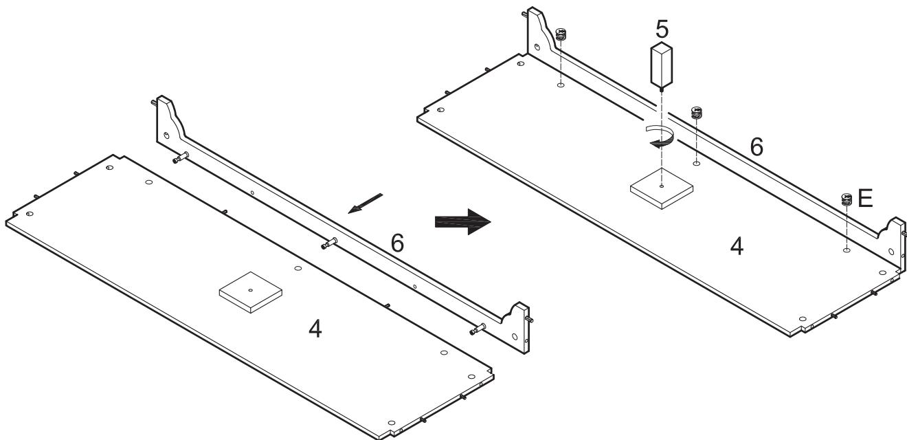
Attach slat (6) to bottom panel (4) using cam bolts and dowels as guides. Insert cam locks (E) into bottom panel (4) and tighten with a screwdriver. Screw leg (5) into bottom panel (4).
