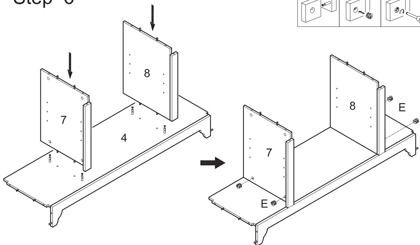
Attach panels (7,8) to bottom panel (4) using cam bolts and dowels as guides. Insert cam locks (E) into panels (7,8) and tighten with a screwdriver.
