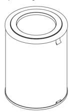
4 Place the filter into the purifier body.
