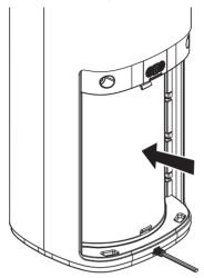
5 Insert the bottom of the filter cover into the purifier housing, then press the top of the cover to snap it into place.
