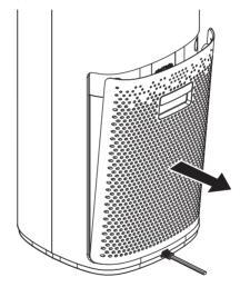
3 Pull the tabs on the top and bottom of the filter to remove it.
