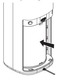
6 Insert the bottom of the filter cover into the purifier housing, then press the top of the cover forward to snap it into place.
