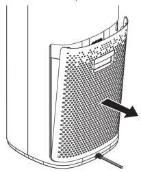
3 Remove the protective plastic bag from the HEPA filter.
