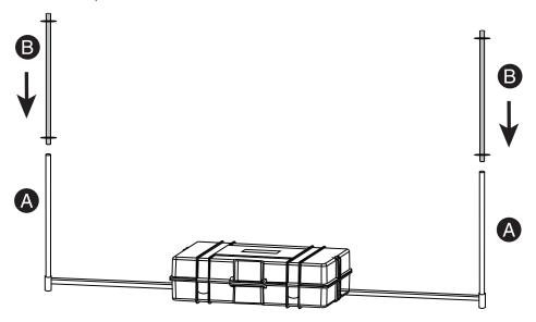
6 Insert an A pole into each B pole.
