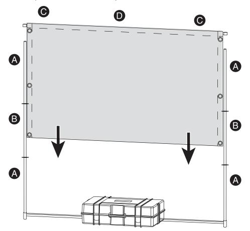
11 To secure the screen to the poles, insert a bungee cord through the grommet on the screen, wrap it around the pole, then insert the plastic ball through the loop on the cord. Attach the other five cords.
