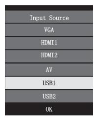
4 Press ▲ or ▼ to on the remote or projector to select the video source, then press OK. You can select VGA, HDMI1, HDMI2, AV, USB1, or USB2.
