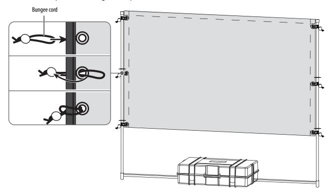
12 To secure the screen to the ground, attach the hook at one end of the string to the hole midway up the B poles. (We recommend that you attach to the holes furthest up the pole.) Attach the hook at the other end of the string to the ground stake. Repeat until all four strings are attached to the poles and stakes. Step firmly on the stakes to insert into the ground. Make sure that the strings are taut and there is no slack.
