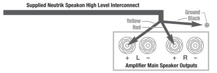
**NOTE:** Classic 99 models are equipped with internal circuitry to allow connection to many Class D (digital) amplifiers.
