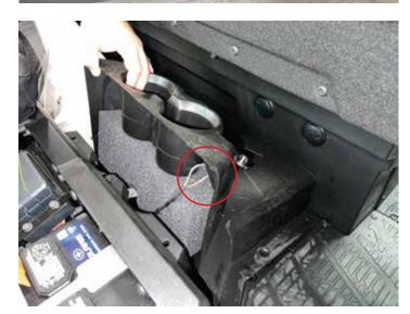
Remove (4) clips from passenger side of front console and (3) clips from driver side. There is (2) hidden clips in center console & if Northstar disconnect front AC hose There is (1) clip hidden behind the fuse holder near the battery.
