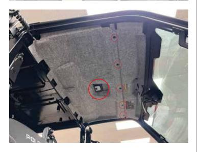
• Unclip rear view mirror harness from roof panel.
