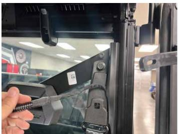
Remove (1) T27 bolt from front driver and (1) T27 bolt from passenger side of roof. Remove the speed clip under the roof (as it will not be needed anymore).
