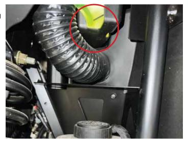
Bring harness up through hole near reservoir (being careful with connector ends). Zip tie to a harness under hood so it doesn't fall back down the reservoir hole.
