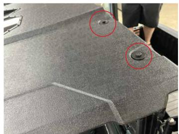
Make sure roof panels are centered properly and go back and tighten all mounting hardware.
