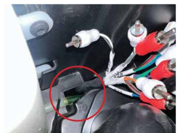
Fold over main harness and push it through the large grommet in firewall that goes into the radio cavity. Carefully bring all the connectors into the radio cavity from the under hood area.
