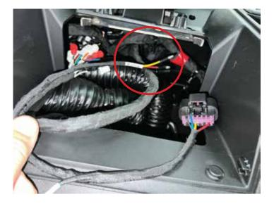
Connect radio harness pulse connectors to the pulse adapter and plug it into the Pulse network module.
