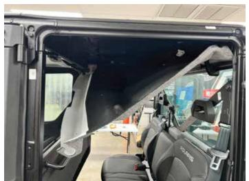
Remove two sections of front headliner. Depending on year and model, you might find push pin clips, dome lights, and T25 or T40 bolts.
