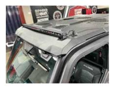
• Bolt front of roof loosely through the lightbar rear bracket hole.
