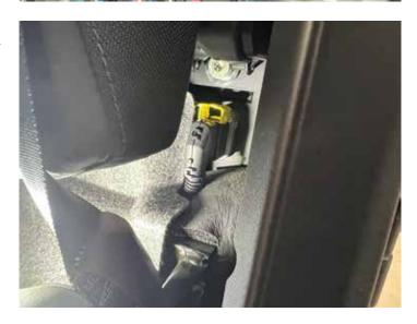
Disconnect power and ground terminals from Pulse network module using a 10mm socket.
