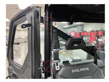
Run harness down by side of seat and behind the carpet panel that is visible between the seat back and seat bottom.
