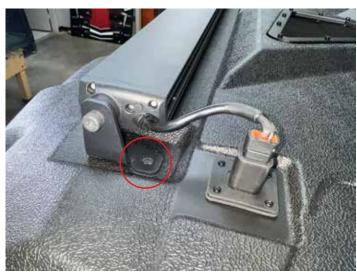
Bolt front and rear sections together using supplied hardware and bracket that goes around the center ROPS bar.
