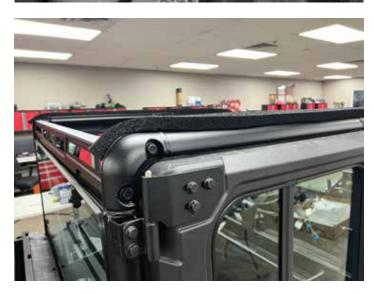
Place rubber gasket in groove on rear cover panel. Loosely install with (4) M6x25 bolts with metal and rubber washers that came in the roof hardware package. Then set rear roof section on top of vehicle.
