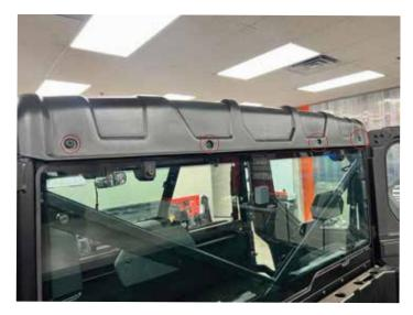
Pull back on rear bottom section of roof while lifting roof and resting on top of ROPS. Then push roof forward and remove.
