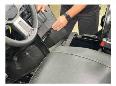
• If you have a windshield, remove (3) T40 bolts and (2) push pin clips in the cup holder panel and set panel aside.
