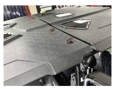
Run main audio roof harness down the passenger rear ROPS pillar and secure with (2) fir tree zip ties in the holes in the ROPS. Leave zip ties loose so you can adjust the wire length during install. You will tighten these later.
