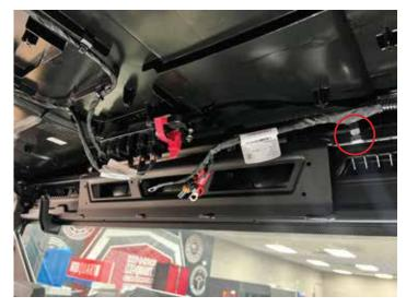
Pull harness out of rubber channel on rear pillar and remove from vehicle or tuck behind rear seat panel.
