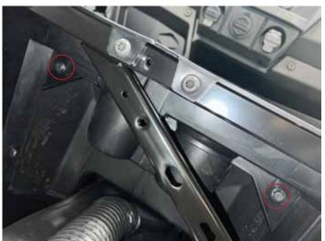
Disconnect air vents from front console then remove front floor console from vehicle.
