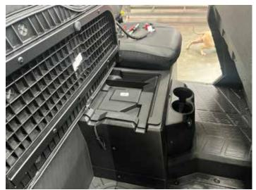
Remove (4) clips from passenger side of front console and (3) clips from driver side. There are (2) hidden clips in center console and if you have the Northstar model disconnect front AC hose. There is (1) clip hidden behind the fuse holder near the battery.
