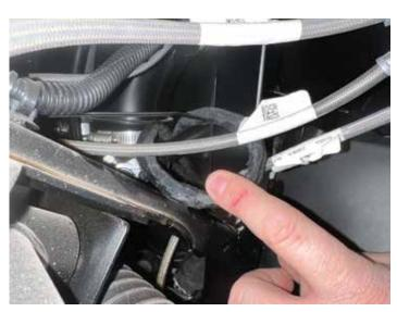
Pull the harness along the firewall and over the brake booster (avoiding all moving parts). Zip tie the harness to a vehicle harness or brake line away from moving parts. You will send it up through the hole where you can see the radiator fluid reservoir.
