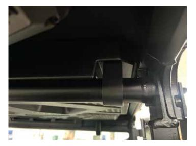
Bolt rear roof section with (4) bolts into the rear cover panel and rear ROPS.
