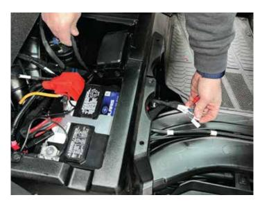
Run harness along factory wiring all the way up to the firewall. Zip tie to white tape marks.
