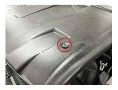
• Remove (4) T40 bolts from rear of roof.
