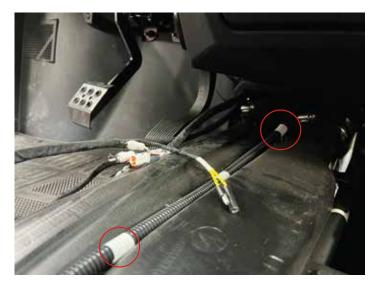
Run harness through firewall on the driver side of opening.
