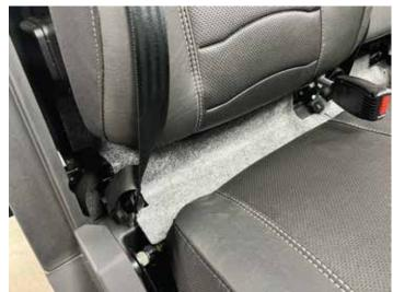
Reach up behind battery and feel for a good spot, between the top and bottom seat pads, to drill a 1 1/8"(29mm) hole to pass the wire harness through.
