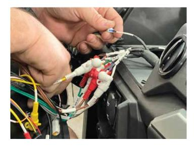
Connect fuse holder to main power wire. Now connect power and ground wires to battery. Now test the system.
