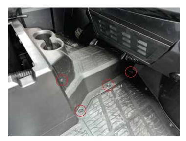
Remove (2) hidden clips from behind front floor console cup holders and disconnect AC hose if it is a Northstar.
