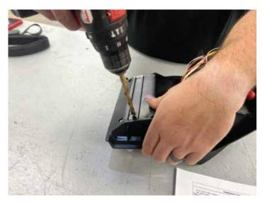
Install radio. Connect the harness that you ran in the previous steps to the connections on the back of the radio.
