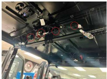
• Disconnect power connector behind driver side seat. Lift yellow clip to unhook connector.
