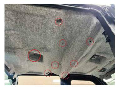
Once all fasteners are removed from the rear headliner, pull the front edge down toward the seats and remove headliner from the vehicle.
