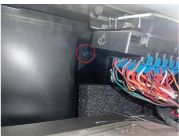
• Lift rear console and disconnect power wort connectors. Remove console from vehicle.
