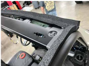
• Side foam should roll over the back of the ROPS by a couple of inches.
