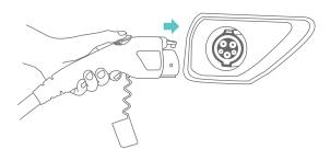
5. When your vehicle is fully charged, the Charging Indicator light will stay solid. Your vehicle has a "dashboard gauge", which also shows if your vehicle is fully charged. Refer to your vehicle user manual to find the location of the gauge on the dashboard.
