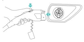
**NOTE:** The charger requires a 120 V AC split phase. It draws a maximum of 15 Amps of continuous current.
