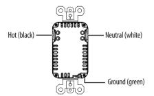
Insert the straightened wire into either of the two holes of the hot and neutral locations on the side of the outlet. Power passes between the two corresponding holes for pass-thru wiring. Attach the ground wire to the bottom of the outlet.
