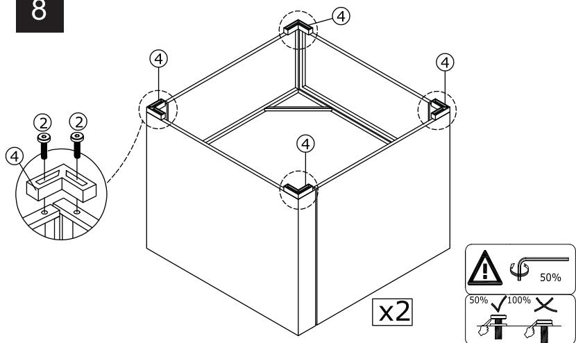
**EN** Connect Part from STEP 7 with Plastic feet (4) & Bolts (2)
