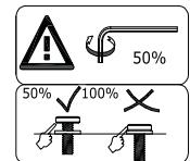
**EN** Connect Big Corner Frame (D) to Small Corner Frame (E) with Bolts (1) & Washers (3)
