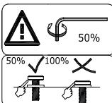
**EN** Connect Side Frame (C) to Corner Seat Frame (F) with Bolts (1) & Washers (3)
