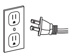
**MARNING**: It is normal for the power cord to feel warm to the touch. However, a loose fit between the outlet and the plug may cause overheating of the plug. If this occurs, try inserting the plug into a different outlet. Contact a qualified electrician to inspect the original outlet for damage.
