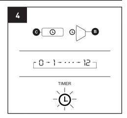
To set the timer power on, while powering off the unit press the Timer button on the control panel (C).
