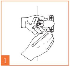
Select an installation location, ensuring that it is a spot that will allow for maximum sun light exposure. Using the wall mount as template mark in the screw holes with a pencil.
