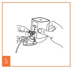
Plug the charging cable into the power connector on Ring Spotlight Cam. Secure the plug with the included screws to keep the connection weatherproof.
