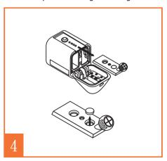
Open the battery compartment of the Ring Spotlight Cam and slide the mounting plate out of its slot. Push the weatherproof rubber plug out of its hole on the mounting plate and return the plate back onto the camera.
