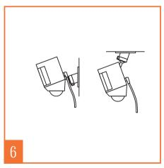
Insert the Ring Spotlight Cam into its mounting bracket and adjust the camera to your desired angle.
