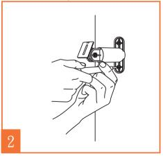
Drill two holes at the position previously marked. Place the included plastic anchor into the hole. Attach the mounting arm to the wall with the screws provided.
