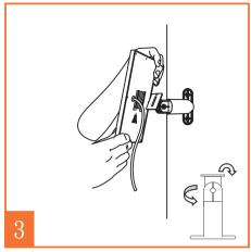
Slide the solar panel onto the wall mount. Adjust and rotate the angle of the Solar Panel for optimum sunlight coverage.
