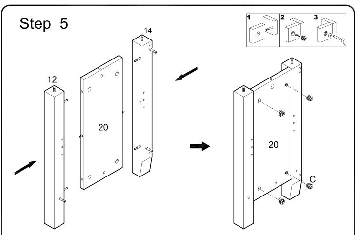
Attach legs (12,14) to second panel (20) using cam bolts and dowels as guides. Insert cam locks (C) into panel (20) and tighten with a screwdriver.
