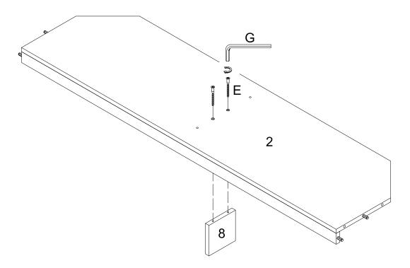
Attach support leg (8) to panel (2) using bolts (E). Tighten bolts (E) with wrench (G).
