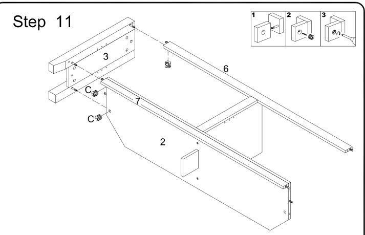
Attach panel (3) with legs (11,13) to the assembly from the previous step using cam bolts and dowels as guides. Insert cam locks (C) into panel (2) and slat (6) and tighten with a screwdriver.
