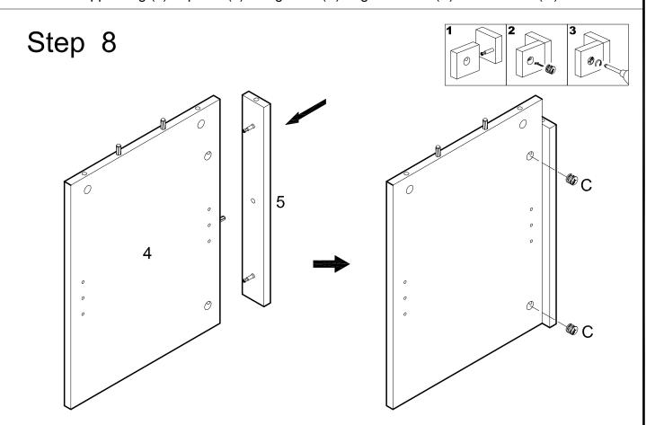
Attach slat (5) to panel (4) using cam bolts and dowel as guides. Insert cam locks (C) into panel (4) and tighten with a screwdriver.
