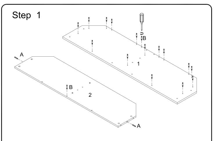
Insert dowels (A) into panel (2). Screw cam bolts (B) into panels (1,2).
