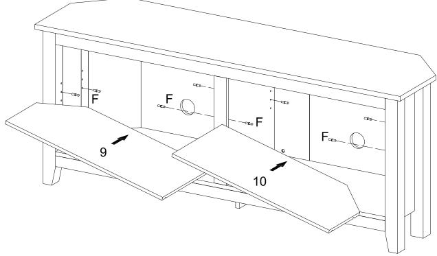
Insert shelf support pins (F) into the assembly at desired shelf heights. Carefully place shelves (9,10) on shelf support pins (F).
