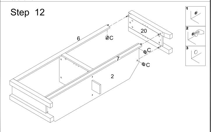
Attach second panel (12) with legs (12,14) to the assembly from the previous step using cam bolts and dowels as guides. Insert cam locks (C) into panel (2) and slat (6) and tighten with a screwdriver.
