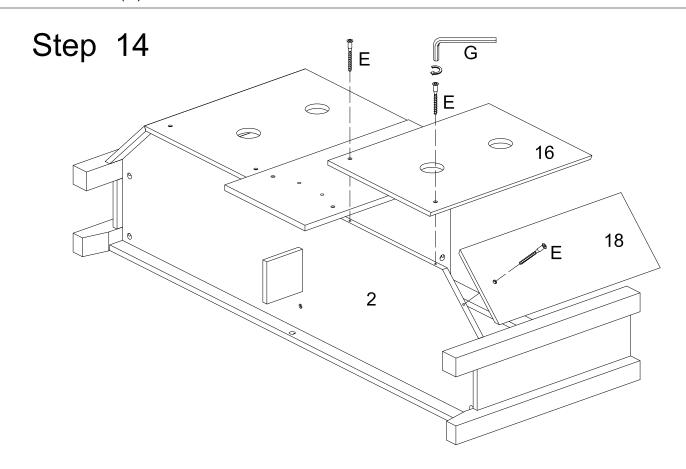
Place the back panel (16,18) on the unit and secure it to the bottom panel (2) with bolt (E) and wrench (G).
