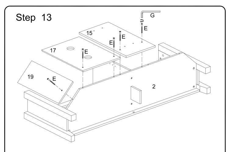
Place the back panel (15,17,19) on the unit and secure it to the bottom panel (2) with bolt (E) and wrench (G).
