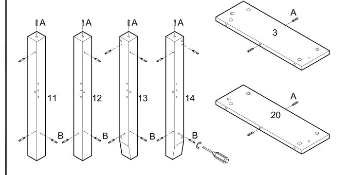
Insert dowels (A) into legs (11,12,13,14) and panels (3,20). Screw cam bolts (B) into legs (11,12,13,14).
