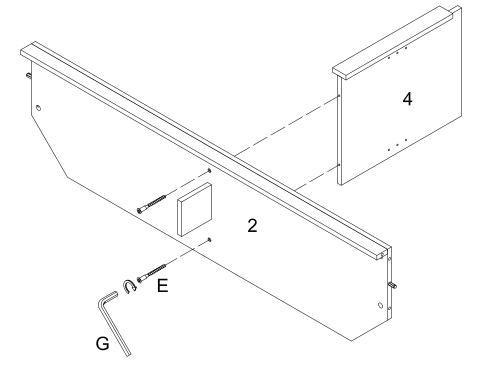
Attach panel (4) to panel (2) using bolts (E). Tighten bolts (E) with wrench (G).
