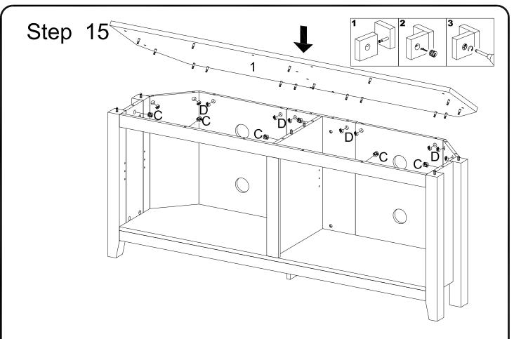
Carefully attach panel (1) to the assembly using cam bolts and dowels as guides. Insert cam locks (C,D) into the assembly as shown above and tighten with a screwdriver.
