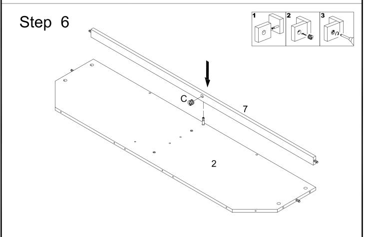
Attach slat (7) to panel (2) using cam bolt and dowels as guides. Insert cam lock (C) into slat (7) and tighten with a screwdriver.
