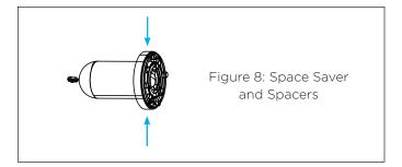
Place the grille aligner around the speaker module and test fit the assembly in the enclosure opening by securing it with two screws (see Figure 8). Test the grille fit. If the grille will not stay on or if there is a gap between the installation surface and the grille, spacers and shims will need to be added or removed until the grille fit is perfect (see Figure 9).
