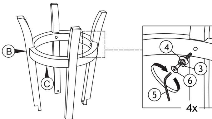
**EN:** Attach each leg (B) to footrest (C). Insert each individual set of hardware as per picture shown. Do not tighten up any hardware completely!
