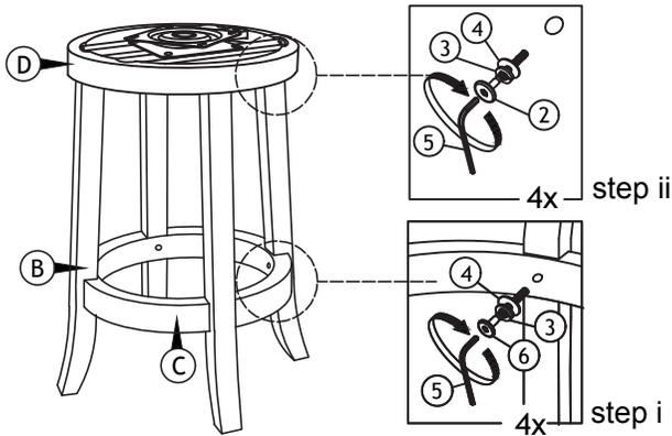
**EN:** Attach each leg (B) to apron (D). Insert each individual hardware as per picture shown. Tighten part(B) with part(C) first, then tighten part(B) with part(D) completely.
