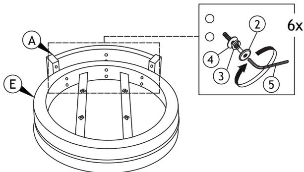
**EN:** Insert 6 sets hardware first, then tighten up part (A) with part (E) together after alignment is done.
