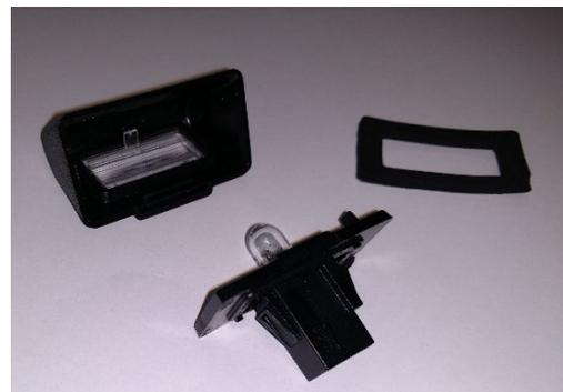
6.) Take the new hood, camera and light diffuser. Make sure the properly line up the factory light fixture with the new hood. Line up the clips to match the factory hood.
