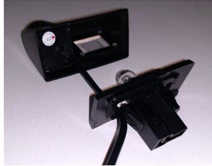
8.) Clip the light fixture back into place. Re-stick the gasket back onto the housing to ensure a watertight fitment.
