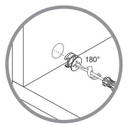
Screw Cam Nut in. Turn clock-wise until you feel Cam Nut securely fasten to Cam Screw. Fully tighten Cam Nut.
