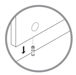
Align hole in panel with Cam Screw.
