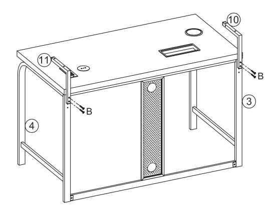
**STEP 5** Secure Left Upper Frame (10) and Right Upper Frame (11) to rear of assembly using two Allen Bolts (B) for each frame. **FULLY TIGHTEN ALL ALLEN BOLTS (B).**
