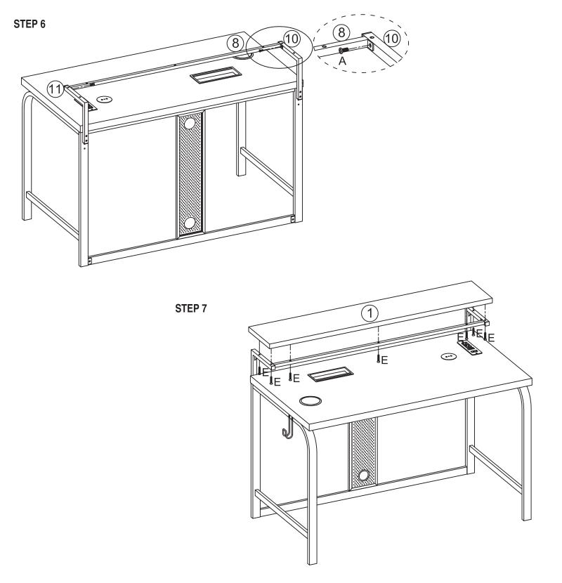
STEP 6 Secure Upper Crossbar (8) between Left Upper Frame (10) and Right Upper Frame (11) using two Allen Bolts (A). FULLY TIGHTEN ALLEN BOLTS (A).
