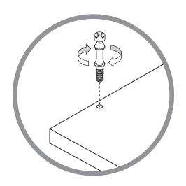
Screw Cam Screw in. Fully Tighten.
