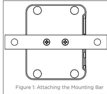
Figure 1: Attaching the Mounting Bar
