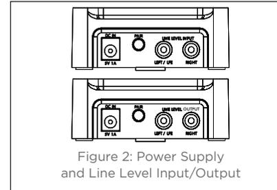
Figure 2: Power Supply and Line Level Input/Output
