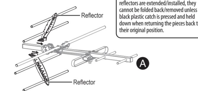
**NOTE:** Once antenna elements and reflectors are extended/installed, they cannot be folded back/removed unless the black plastic catch is pressed and held down when returning the pieces back to their original position.
