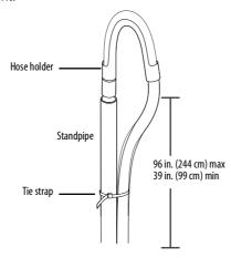
• In a laundry tub - The laundry tub must be no shorter than 39 in. (99 cm) and no higher than 96 in. (244 cm) maximum.
