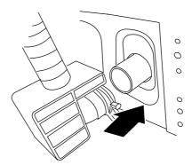
3 Move the clamp toward the drain pipe outlet. Tighten the clamp with pliers.
