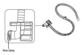
2 Insert the drain hose with the clamp onto your washer's drain pipe. Make sure that the drain hose completely covers the end of the drain pipe.
