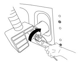
4 Connect the ends of the water supply hoses to the water supply intake connections at the top of your washer. Make sure that the rubber washers are in place. The water supply hose connected to the hot faucet must be connected to the hot water supply intake and the water hose connected to the cold faucet must be connected to the cold water supply intake.
