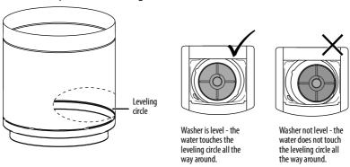
3 If your washer isn't level, carefully tilt your washer just enough to adjust the two leveling feet on the bottom of the front of your washer. Extend the feet only as much as is necessary. If the feet are extended too much, your washer may vibrate.
