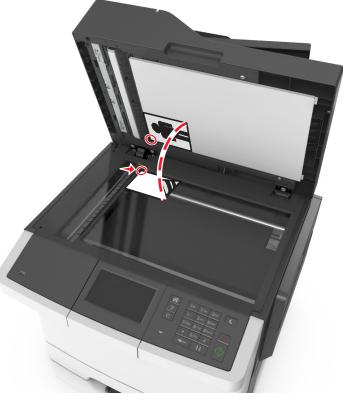
A photograph of the same printer with its scanner glass open. A white sheet of paper is placed on the glass. A red arrow points to the paper on the scanner glass. <p>Use the scanner glass for single-page documents, book pages, small items (such as postcards or photos), transparencies, photo paper, or thin media (such as magazine clippings).</p> |
