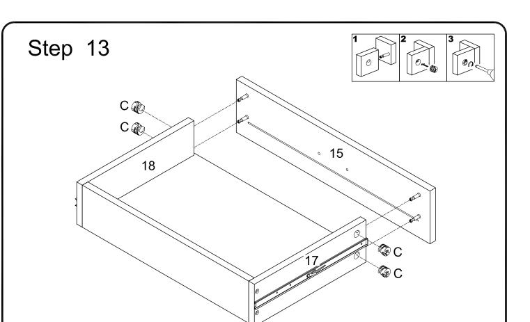
Insert drawer front panel (15) into drawer side panel (17,18), then insert and secure cam lock (C) to drawer side panel (17,18) to lock it.
