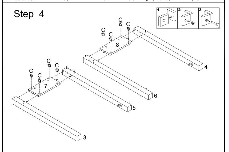
Insert side panel (7,8) into legs (3,4,5,6), then insert cam lock (C) into side panel (7,8) and lock it.
