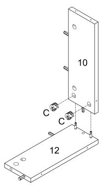
Insert middle side panel (9,10) into front panel (11,12), then insert and secure cam lock (C) to middle side panel (9,10) to lock it.
