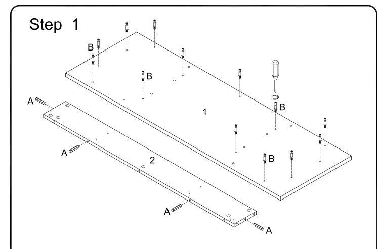
Insert wooden dowel (A) into back panel (2). Secure cam bolt (B) to top panel (1).
