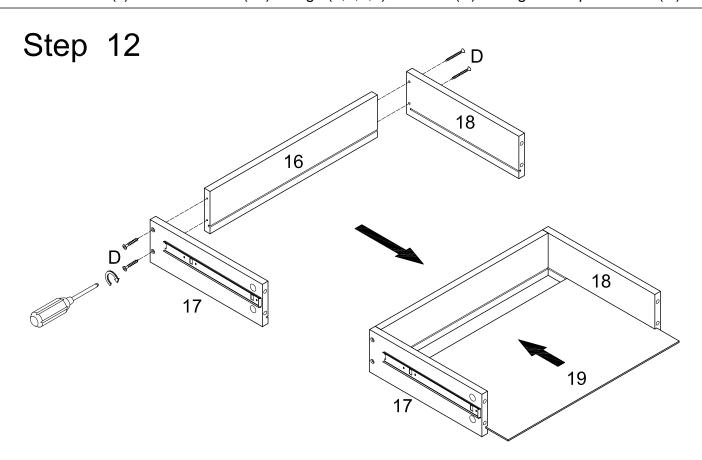
Secure drawer side panel (17,18) to drawer back panel (16) with screw (D). Insert drawer bottom panel (19) through side panel (17,18).
