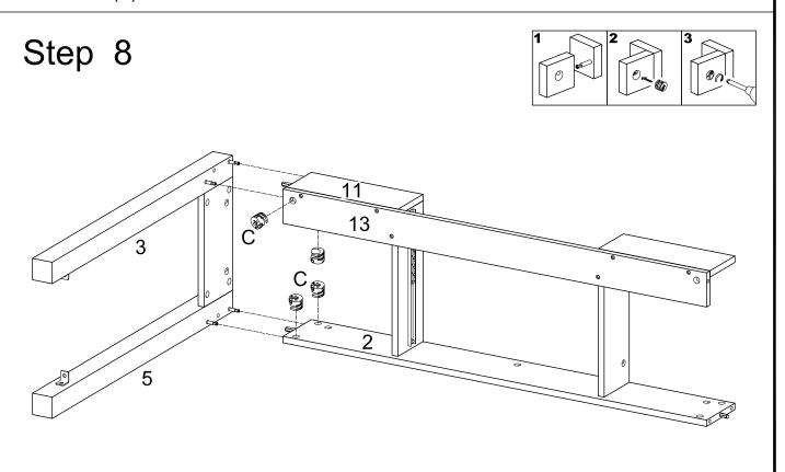
Insert legs (3,5) into drawer front panel (11), bottom support bar (13), and back panel (2), then insert and secure cam lock (C) to drawer front panel (11), bottom support bar (13), and back panel (2) to lock it.
