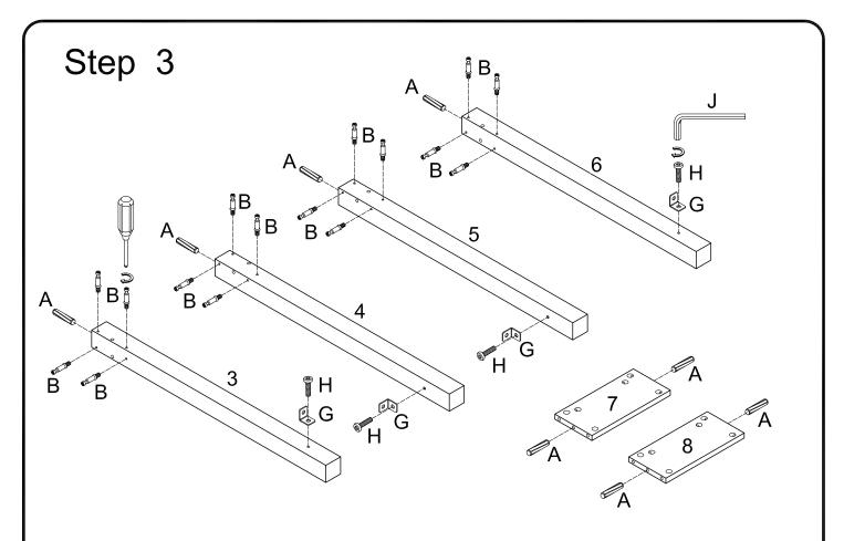
Insert wooden dowel (A) into side panel (7,8), and legs (3,4,5,6). Secure cam bolt (B) to legs (3,4,5,6). Use wrench (J) to secure L shape bracket (G) to legs (3,4,5,6) with bolt (H).
