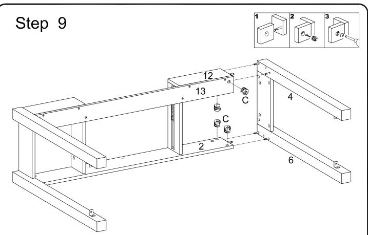
Insert legs (4,6) into drawer front panel (12), bottom support bar (13), and back panel (2), then insert and secure cam lock (C) to drawer front panel (12), bottom support bar (13), and back panel (2) to lock it.
