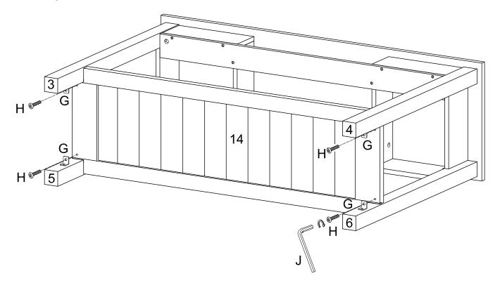
Use wrench (J) to secure shelf (14) to legs (3,4,5,6) with bolt (H) through L shape bracket (G).
