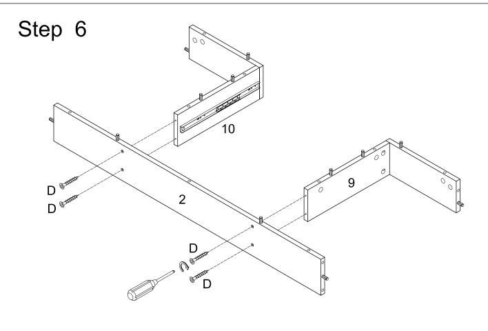
Secure back panel (2) to middle side panel (9,10) with screw (D).
