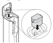
Press the battery down into the compartment.
