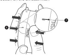
9 Push and insert the exhaust filter cover 3 into the exhaust filter **1** and rotate it to reassemble it and prevent it from falling out.
