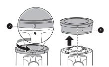
Grip the exhaust filter cover 3 and the exhaust filter **1** using both hands and rotate the exhaust filter cover while pressing the **PUSH** button in order to separate it from the exhaust filter.
