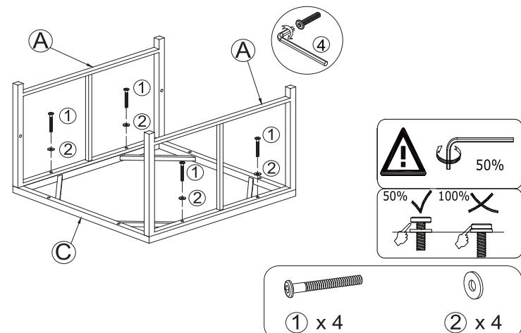
**EN:** Please don't fasten the screw completely during assembly process. It will be likely to lead to an assembling problem that screw hole position is not aligned. You can fasten completely when all parts have been assembled.
