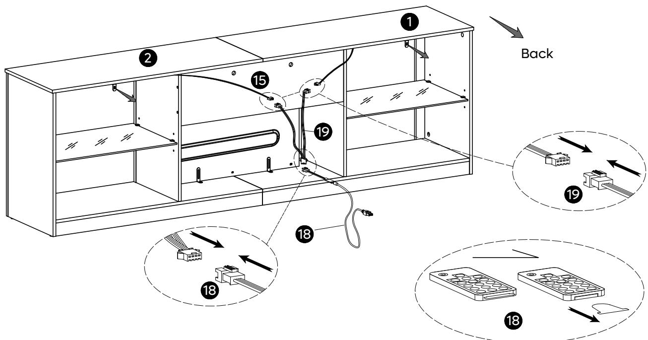
Take out the insulator before using the remote control.
