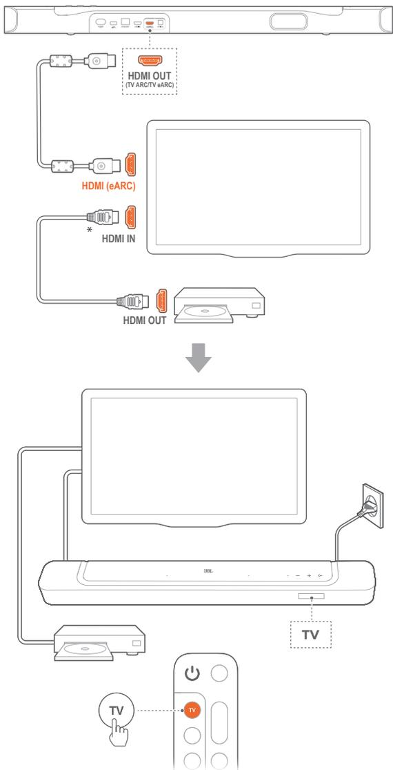
1. Connect the soundbar with the **HDMI IN (eARC)** connector on your TV by using the supplied HDMI cable.
