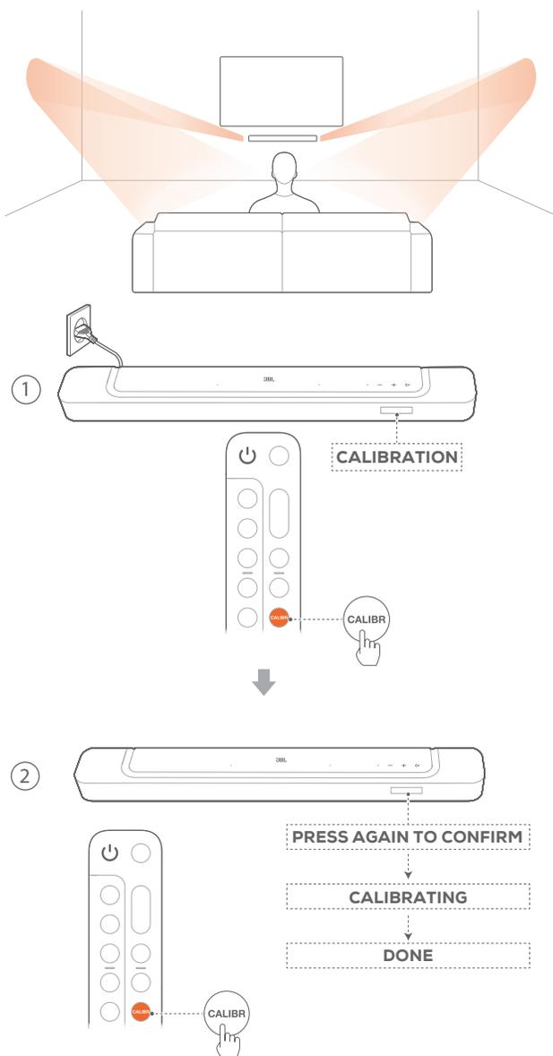
1. On the remote control, press **CALIBR** to start calibration.
