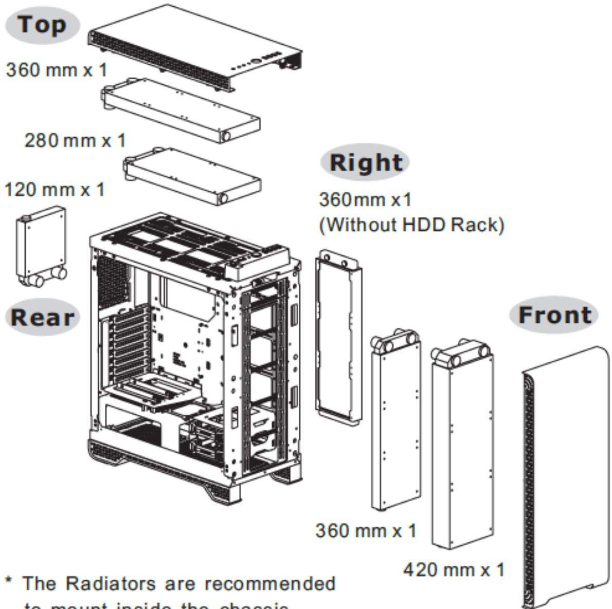
\* The Radiators are recommended to mount inside the chassis.
