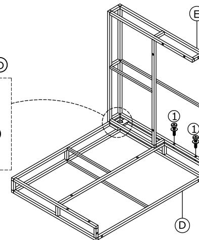
**EN** Connect Big Corner Frame (D) to Small Corner Frame (E) with Bolts (1) & Washers (3)
