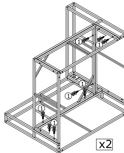
**EN** Connect Part from STEP 5 to Part from STEP 6 with Bolts (1) & Washers (3)
