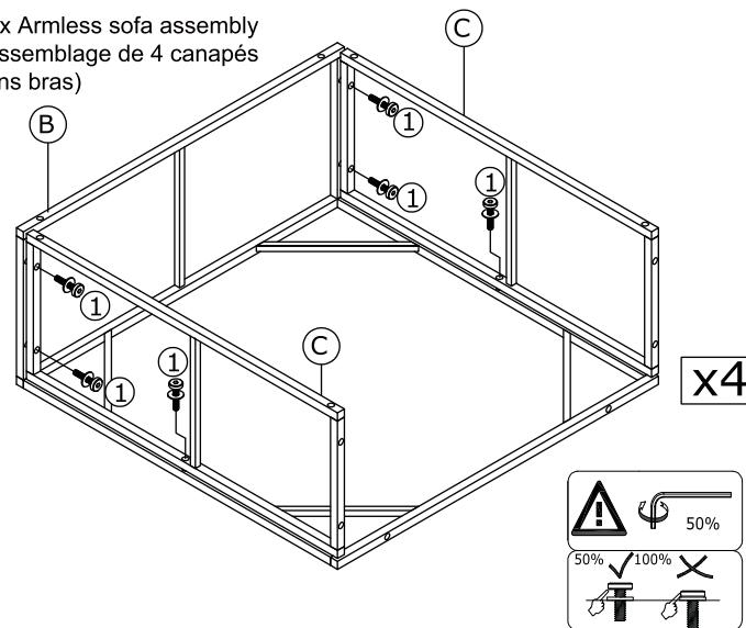
**EN** Connect Side Frame (C) to Seat Frame (B) with Bolts (1) & Washers (3)
