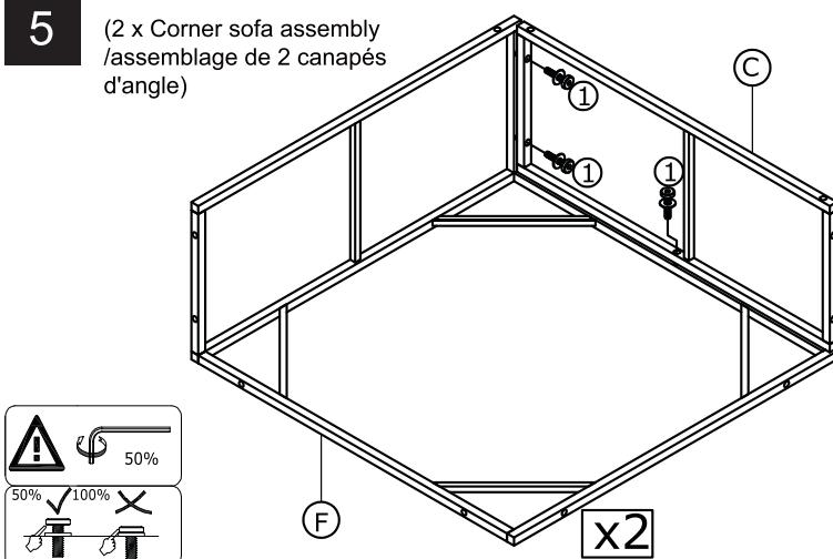
**EN** Connect Side Frame (C) to Corner Seat Frame (F) with Bolts (1) & Washers (3)
