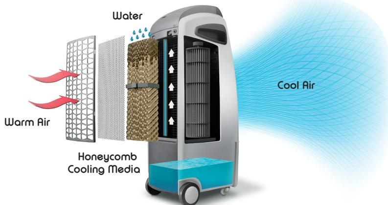
When you add water in the tank, Quilo™ QEIS evaporative cooling technology rapidly reduces the temperature of incoming warm air, creating a refreshing cool breeze. A fan simply recirculates warm air. In Evaporative Cooling mode, the Quilo™ QEIS can rapidly reduce the temperature of incoming warm, dry air through the process of evaporation, creating natural cool air output. Imagine that amazing comfortable cool breeze you feel when standing near a lake or sea.
