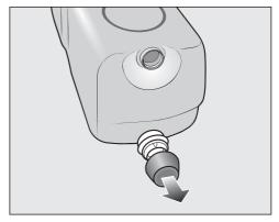
Remove the cover caps from the detergent cartridges included with the delivery.
