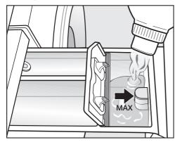
■ Add the fabric softener or the liquid starch to the
