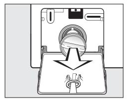
■ Remove the drain filter completely.
