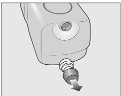
Remove the cover cap from the cartridge.
