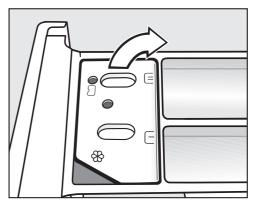
■ Open the lid of the \( \mathre{\pi} / \subseteq \text{compartment.} \)
