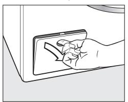
Open the drain pump flap.
