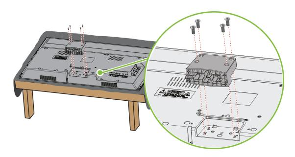
**3** Find the front of the TV stand, then secure the stand to the stand column using the five provided 16 mm screws. (These are the long screws.)
