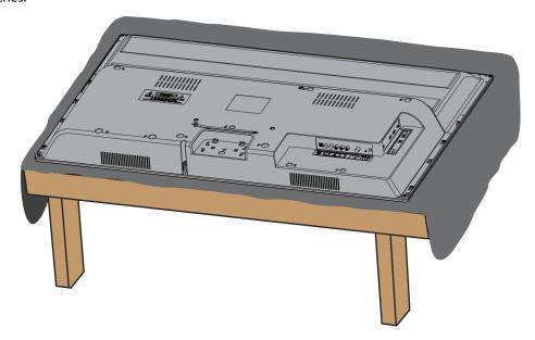
2 If the stand is attached, remove the four screws that secure the stand column to the TV, then remove the stand column.
