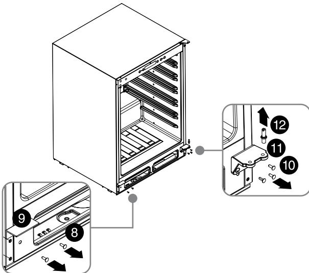
**E** Reinstall the door support (9) and lower hinge (11) on the opposite sides, then place the lower hinge shaft (12) back into the lower hinge.
