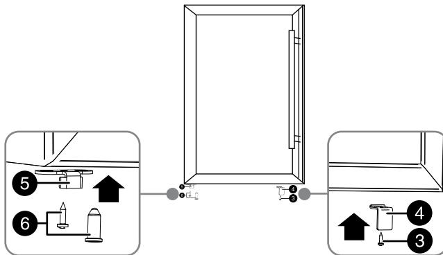
**5** Place the door on the cooler's lower hinge shaft, then secure with the upper hinge bolt (1).
