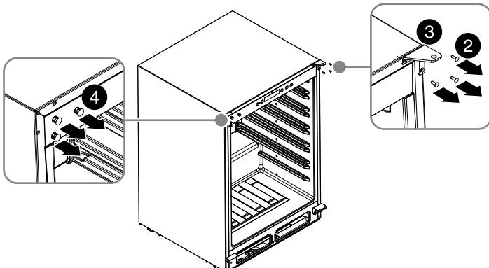
**B** Install the upper hinge from the included accessories bag (3) to the opposite side, then insert the plastic caps (4) into the old screw holes.
