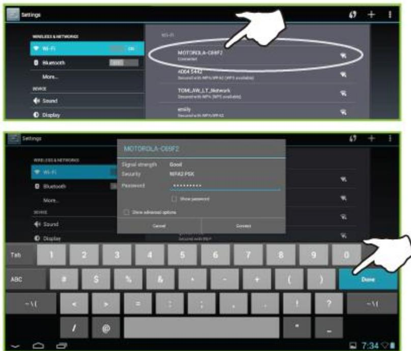
5. Touch **Connect**. A wireless connection icon appears in the lower right-corner of the screen when the connection is successful.
