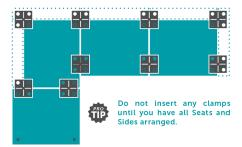
Place two more Seat Frames on the Shoes that are exposed. Again, adjust the Shoes so they are straight and square with the alignment marks. Notice that this configuration will not require Shoes at the end of the chaise ottoman.
