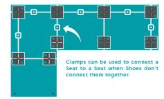
Use the steel Clamp to attach all Sides to the Seat Frames to complete our patented system.
