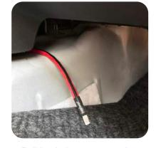
3. Pull back the carpet on the passenger side of the center console and pull the length of wire through to the passenger side.
