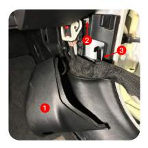
1. Remove the kick panel access cover (1), remove the 10mm nut (2) and unhook the door check strap.
