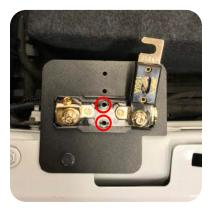
4. Temporarily loosen the 4mm fuse set screws and move the fuse to access the two mounting holes in the base.
