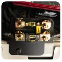
2. X-Link inputs and outputs can accept 0/1, 4 and 8 GA wire. ANL or MIDI fuses can be used, or a combination of both as shown above.
