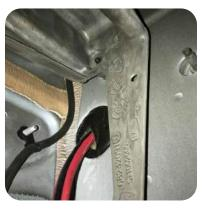
6. Inside the vehicle, to the left of the brake pedal, pull the lenght of the power wire into the vehicle.
