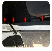
2. Starting at the front, pull the kick/door sill panel towards the center of the vehicle to release the retaining clips and remove.
