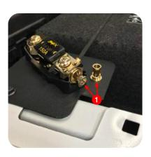
3. If installing the 4GA kit, remove the 8GA inserts (1) from both ends of the fuse holder by losening the 4mm wire set screws.
