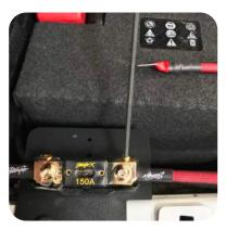
1. Using a 4mm allen, securley connect the ferrule end of the 22in Fuse to Battery cable to the right side of the fuse holder. Route the eyelet end to the posive battery terminal.
