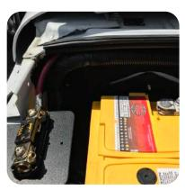
1. Starting at the fuse, route the power wire along the factory harness running across the rear of the engine compartment.
