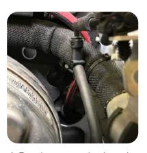
9. Run the power wire through the grommet and into the vehicle. Reinstall the plastic insert in the firewall.
