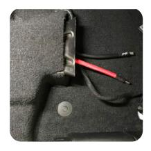
9. Route the ground wire under the carpet and out the air vent opening.
