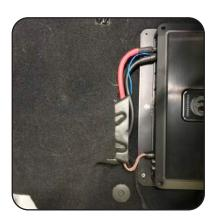
1. At this point, the amplifier should be set in place. If using an amp mounting bracket, the amplifier should be attached to the bracket and then set in place. For each connection, ensure there is the proper amount of wire lenght.
