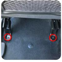
2. Move the seat to the front and remove the two rear Torx T50 seat bolts.
