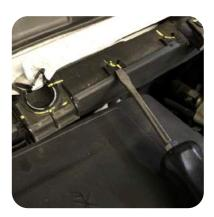
4. Starting on either side, use a flat blade screwdriver to release the locking tabs along the top of the wire cover.
