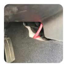
2. Pull back the carpet at the front of the center console on the driver's side. Feed the power wire across to the passenger side.
