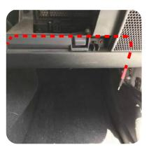
5. Route the power wire across the glove box opening following the factory wire harness. Secure with zip ties.
