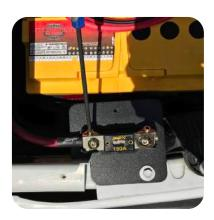
7. Insert the braided sleeved end of the XX power cable into the left side of the fuse holder and tighten the 4mm set screw.
