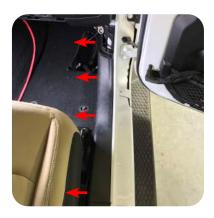
4. Remove the kick/door jamb panel by pulling it towards the center of the vehicle.
