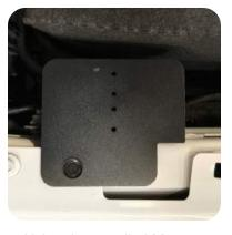
2. Using the supplied M6 x 25 bolt attach the fuse mounting plate in the direction shown above.
