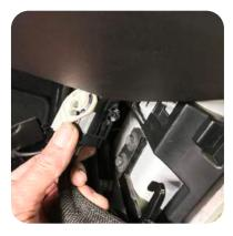
2. Using a trim tool, unclip the electrical connector from the body.
