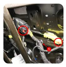
3. Tilt the seat back and disconnect the two electrical connectors on the bottom. Unclip the wire harness (1).
