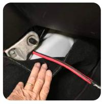
4. Unsnap and pull back the carpet on the passenger side of the center console and pull the lenght of wire through to the passenger side.
