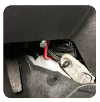
3. Unsnap and pull back the carpet at the front of the center console on the driver's side. Feed the power wire across to the passenger side.
