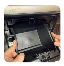
4. Remove the glove box by pushing inward on both sides and lowering to unhinge the bottom.
