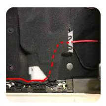
7B. DRIVER SIDE: Route the power wire down from the upper dash area to the kick panel harnesses, then along the door jamb, and finally out under the seat through the air vent opening.
