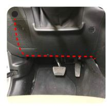
2. If mounting the amp under the passenger seat, route the power wire across the lower dash. Follow the factory wire harnesses and secure with zipties.
