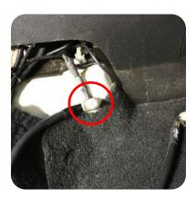
8. On both sides of the console there will be a factory ground point. Remove the 10mm nut and attached the Black 12in Ground lead. Retighten the nut securely.
