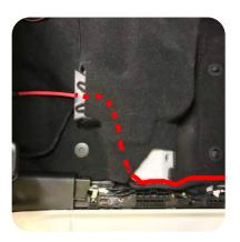
7A. PASSENGER SIDE: Route the power wire down from the glove box area to the kick panel harnesses, then along the door jamb, and finally out under the seat through the air vent opening.
