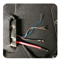
3. Route the RCA cable and the terminated end of the blue Remote Turn On wire under the carpet from the side of the center console to the air vent opening.
