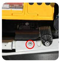
1. The fuse mounting plate will be attached to the passenger side fender near the battery using the 10mm bolt indicated.
