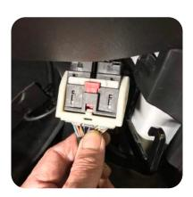
3. Disengage the red lock and disconnect the connector.
