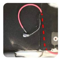
6A. PASSENGER SIDE: Route the power wire down from the glove box area to the kick panel harnesses, then along the door jamb, and finally out under the seat through the opening in the carpet.
