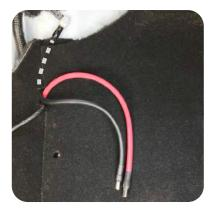
8. Route the ground wire under the carpet and out the opening in the carpet.
