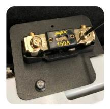
6. Reinstall the fuse and tighten the set screws.
