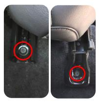
1. Move the seat to the rear and remove the two front Torx T50 seat bolts.
