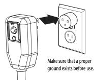
To prevent damage to the adapter's ground terminal, hold the adapter in place while plugging or unplugging the air conditioner.
