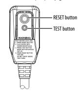
The circuit breaker should be tested periodically by pressing the **TEST** button, then pressing the **RESET** button. If the **TEST** button does not cause the circuit breaker to trip, or if the **RESET** button does not stay engaged, unplug the air conditioner immediately and contact an Insignia technician.
