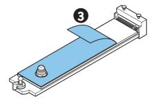
**4.** If you install 22110 SSD, remove the installed **EZ M.2 Clip II** from 2280 screw hole by using the included **EZ M.2 Clip II Remover**. Skip this step if you install 2280 SSD.
