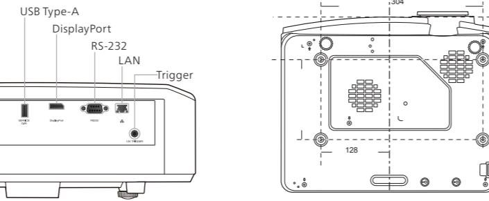
External Dimensions (W x D x H): 405 mm x 341 mm x 146 mm (15 • 7/8" x 13 • 1/2" x 5 • 3/4")
